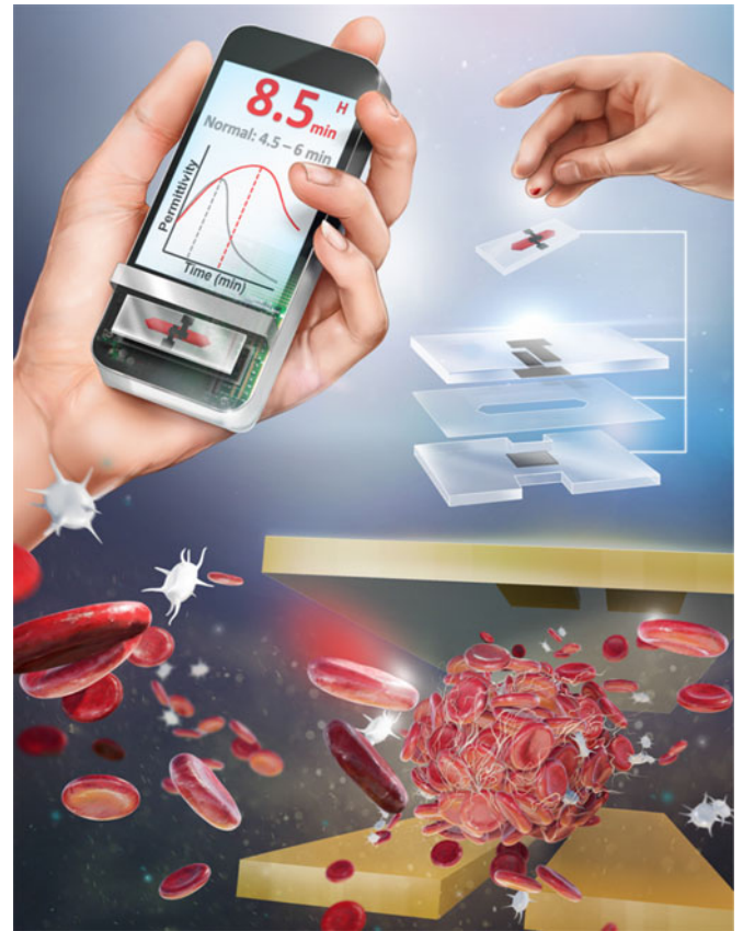
Fig. 1. Conceptual illustration of a POC dielectric coagulometer utilizing the proposed ClotChip microfluidic sensor.
